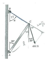
2. For the frame and loading shown, determine the components of the forces acting on member ABC at B and C. (25%)
