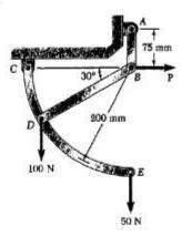
Determine the range of values of force P for which equilibrium of the block is maintained. (25%)
